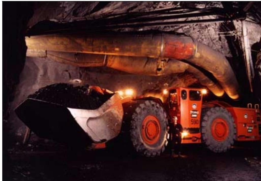
25 to 30 loaders are rolling in triple-shift in Europe's largest and smallest iron ore mines. These machines are driven by skilled personal that manoeuvre the beasts in narrow drifts at high speed. The largest machine weighs 80 tons and has a bucket capacity of 25 tons. Some rumours say that the record is in excess of 50 tons, yet this has not been confirmed, but it is not totally unbelievable.
