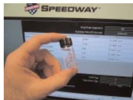
Figure 2 Monza-driven item-level tags read even inside a water-filled vial.
